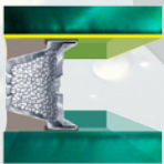
Double Glazed Tempered/Tempered
