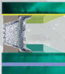
Double Glazed Tempered/Laminated
