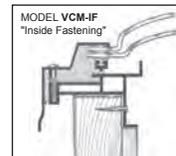
Now you are ready to install your Columbia Skylight. Apply 1/2" thick continuous bead of non hardening caulking or foam tape on the top of the roof curb. Set the skylight firmly onto the curb. If it doesn't fit easily, recheck curb dimensions and squareness then make any adjustments.
