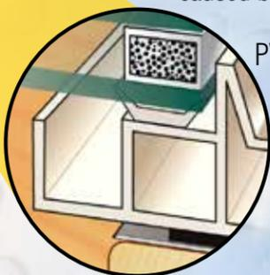
PVC (Polyvinyl Chloride) Base Frame with effective 4-sided rigid condensation gutter
