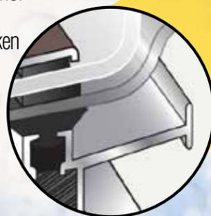
Thermally broken Aluminium Base Frame with effective 4-sided rigid condensation gutter
